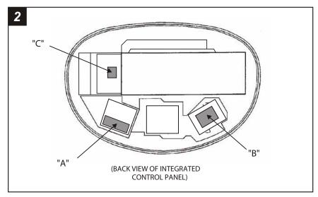
Turn the integrated control panel over and disconnect the vent control harness ("A"), fan speed control harness ("B"), and defroster harness ("C"). Unclip the main switch harness from the side of the factory unit. (This harness connects the fan speed control harness, vent control harness and defroster harness).
